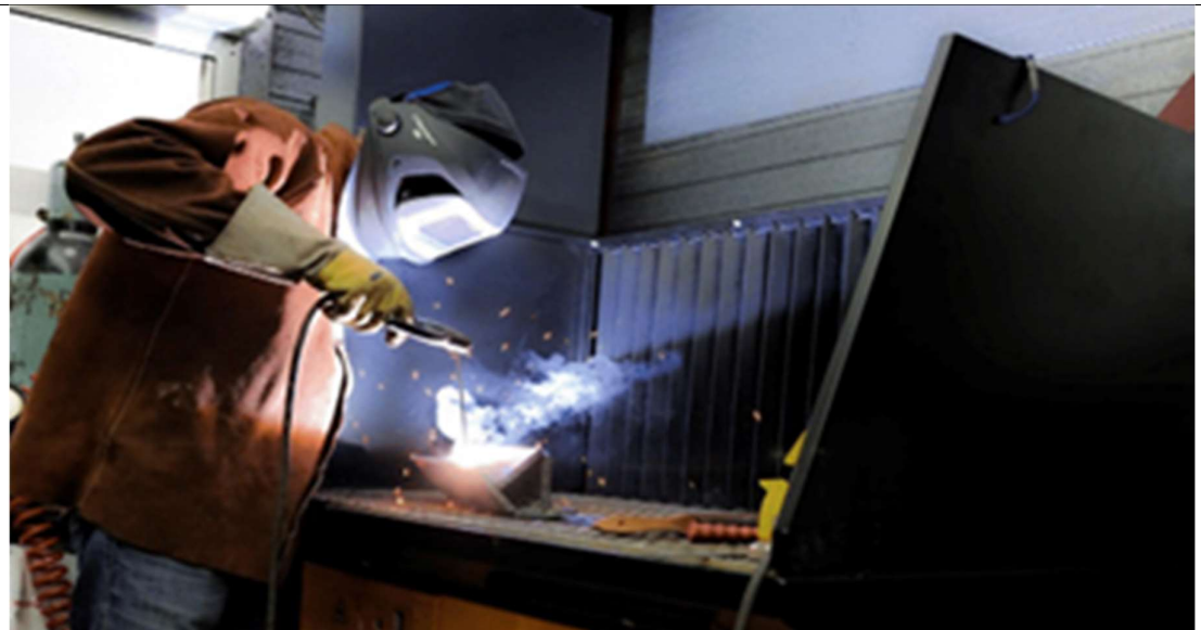
Photo 2 Good control practice - MMA with an effective welding bench (RPE also required) (Plymovent, GB)
