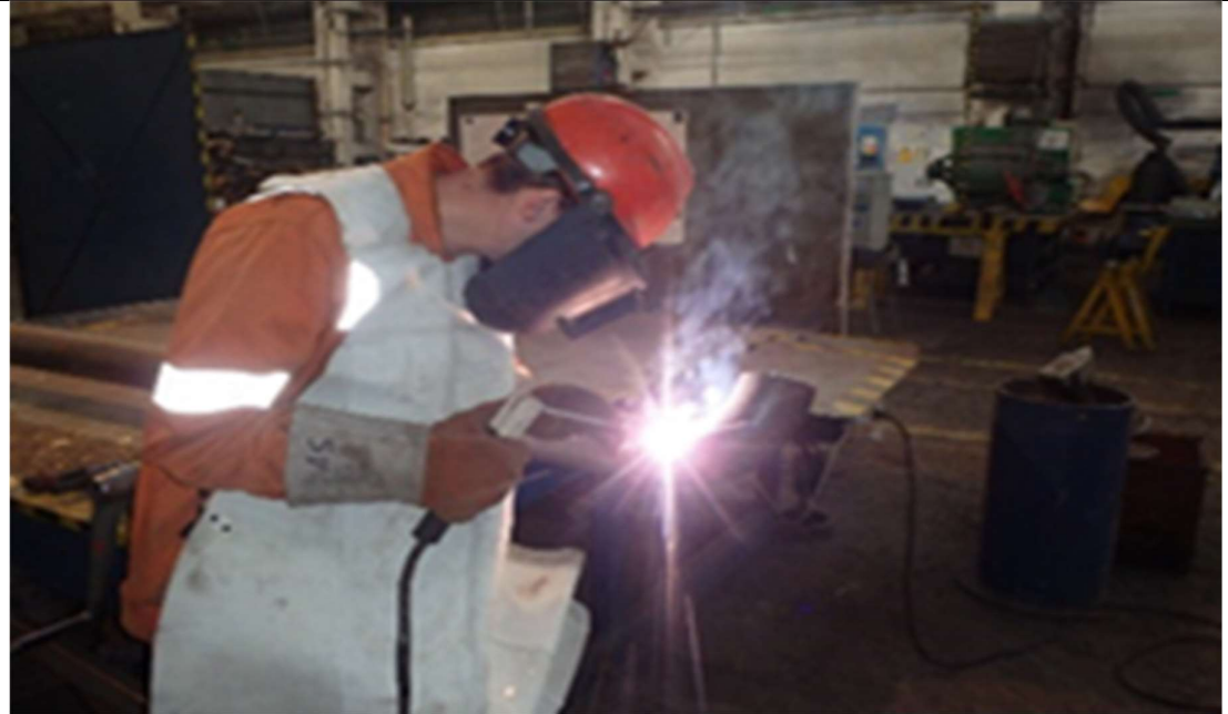
Photo 1 Poor control practice - MMA without LEV (NLI, SK)
